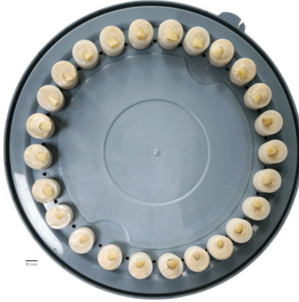
Placement of Samples in the Smoke Chamber
